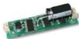
Fig. 4: Power management circuit to regulate and store the harvested electrical energy (Advanced Linear Device, INC, 2011).
