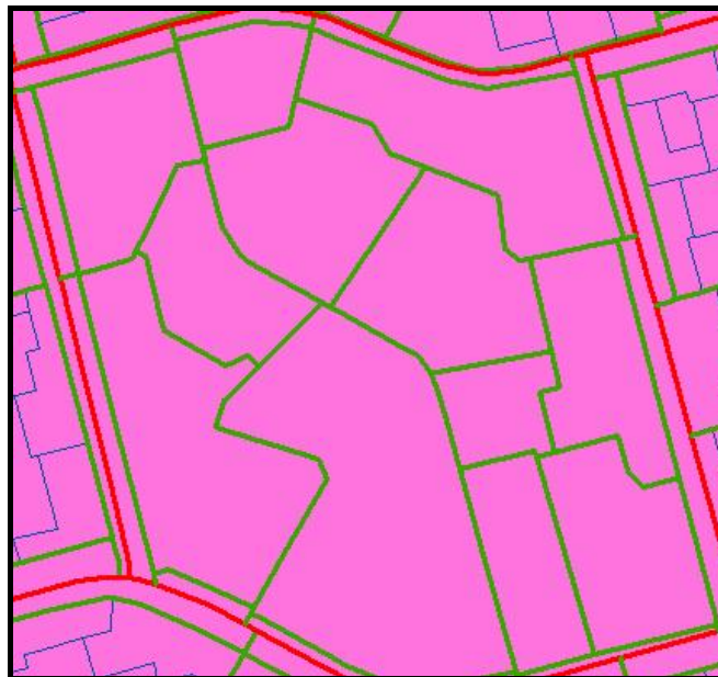
Fig. 3: Completely loop network with service pipes equal to or greater than 200mm.
