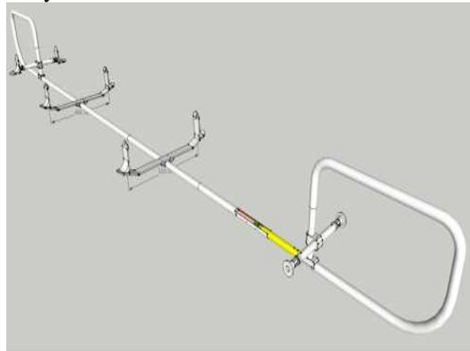
**Fig. 7:** 3D modeling of Frame structure of a frame-type small boat.
