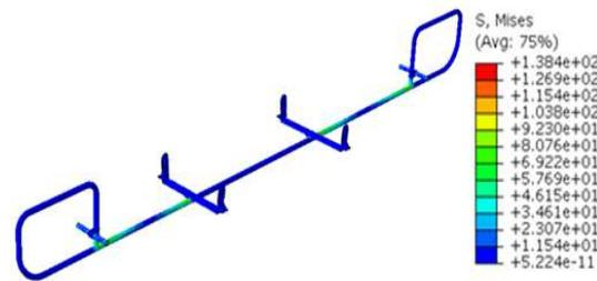
**Fig. 12:** Strain of frame when 1 person got on board.
