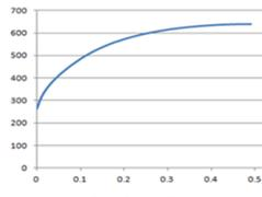
SUS304 True Stress-True Strain test |             |
