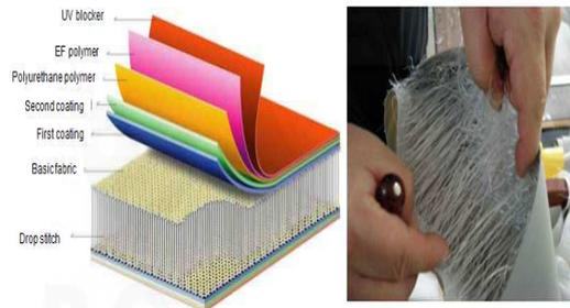
**Fig. 1:** Configuration and inside shape of extra-high-pressure space paper.
