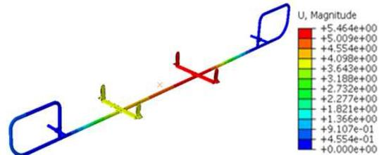
**Fig. 13:** Stress distribution of frame when 1 person got on board.
