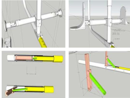
**Fig. 6:** Length adjustment system for implementation of adjustment of angle and height of a boat and convenience of disassembly.
