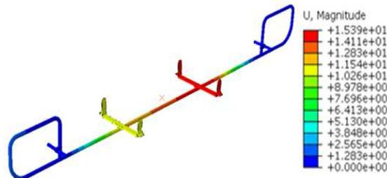
**Fig. 14:** Strain of frame when two people got on board.
