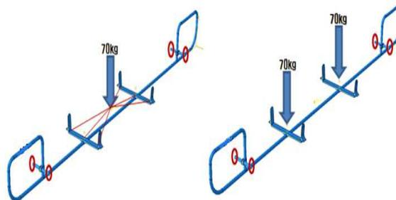
**Fig. 10:** Boundary/load conditions when one or two adults got on board.
