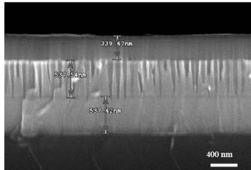
**Fig. 7:** FESEM image after improving etch profile
