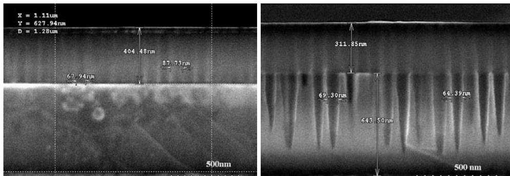
**Fig. 6:** FESEM cross-section views of the sample : (a) before and (b) after etching GaN
