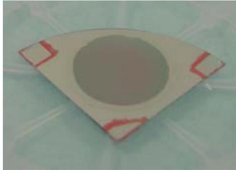
**Fig. 2:** The porous alumina mask on GaN/sapphire
