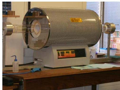
**Fig. 1:** The instruments to fabricate the etch masks: (a) the anodization cell and (b) the tube furnace
