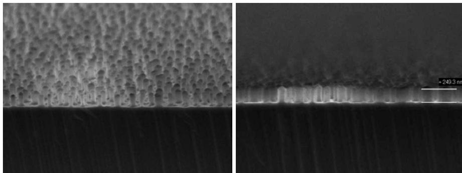
**Fig. 8:** FESEM images of  $\text{SiO}_2$  nano-columns
