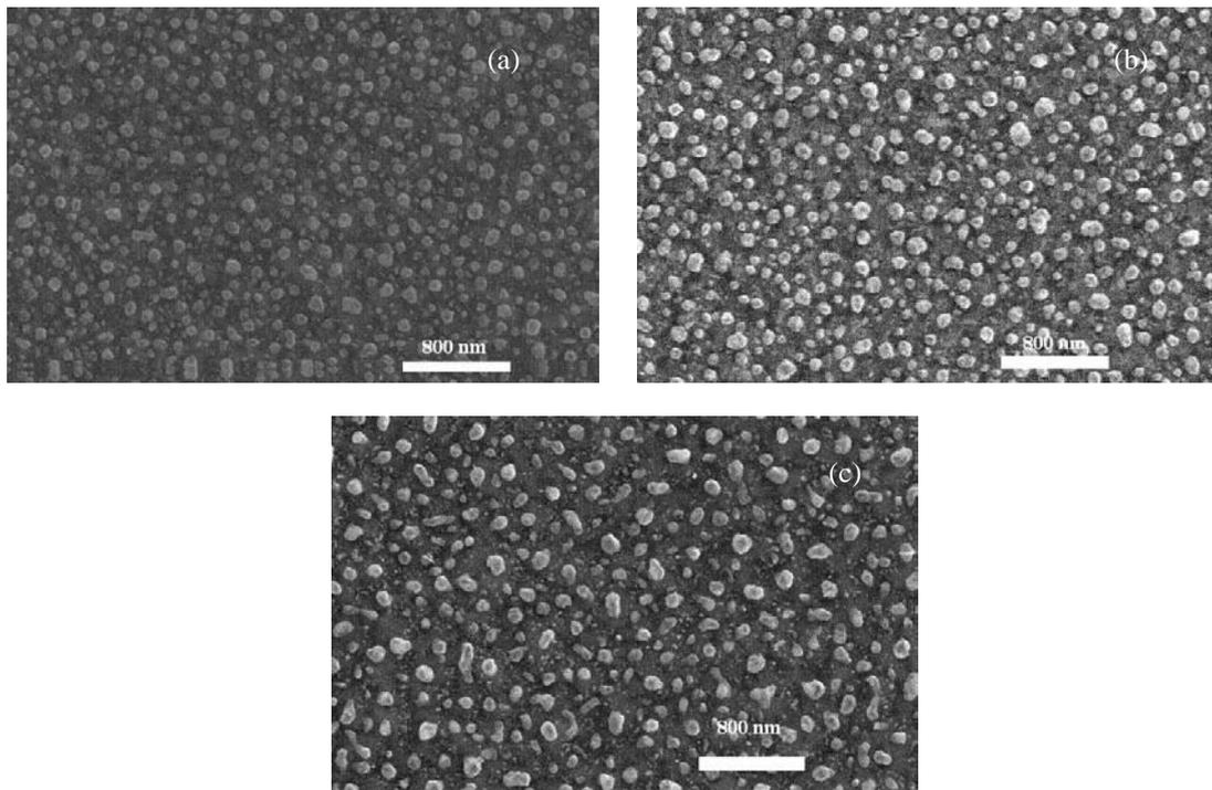
**Fig. 5:** Ni dots formed at 800°C for (a) 30 sec (b) 31 sec and (c) 33sec (Si)
