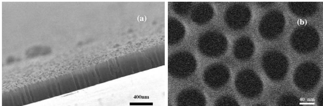
**Fig. 3:** FESEM images of the porous alumina mask : (a) cross section (b) plan-view
