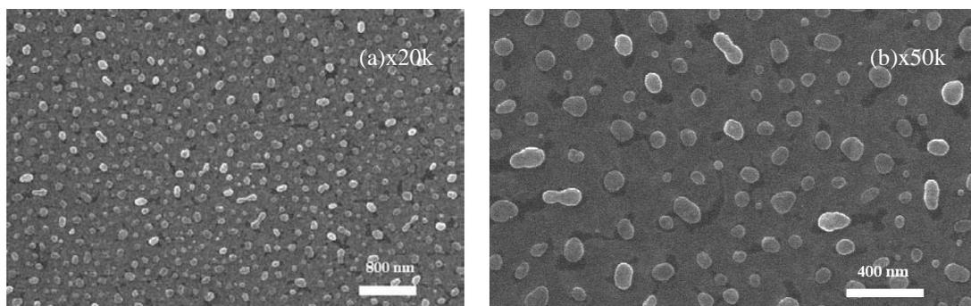
**Fig. 4:** Ni dots formed at 845°C for 45 sec (sapphire)
