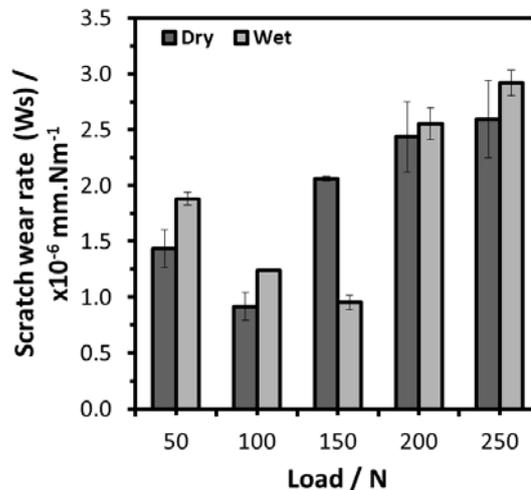
**Fig. 3:** Scratch wear rate at different loads (50 N, 100 N, 150 N, 200 N, and 250 N) under dry and wet condition test.
