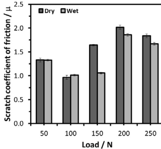
**Fig. 4:** Scratch coefficient of friction at different loads (50 N, 100 N, 150 N, 200 N, and 250 N) under dry and wet condition test.
