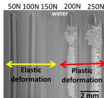
**Fig. 6:** Scratch damage at different loads (50 N, 100 N, 150 N, 200 N, and 250 N) under wet condition test.
