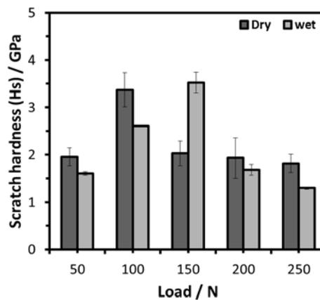
**Fig. 2:** Scratch hardness at different loads (50 N, 100 N, 150 N, 200 N, and 250 N) under dry and wet condition test.
