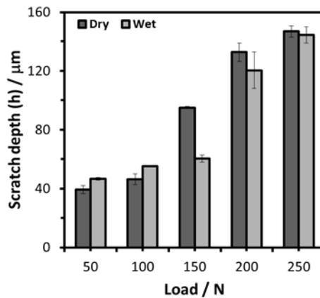
**Fig. 1:** Scratch depth at different loads (50 N, 100 N, 150 N, 200 N, and 250 N) under dry and wet condition test.
