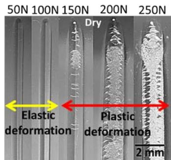
**Fig. 5:** Scratch damage at different loads (50 N, 100 N, 150 N, 200 N, and 250 N) under dry condition test.
