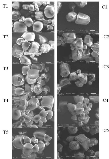
**Fig. 1:** Scanning electron micrographs of microwave heat-treated flour samples (25% w/w) at difference time:
