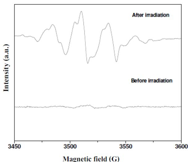
**Fig. 2:** ESR spectra of alanine before and after radiation
