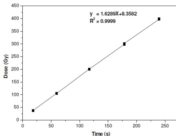
**Fig. 1:** expose time according to radiation dose from Fricke solution
