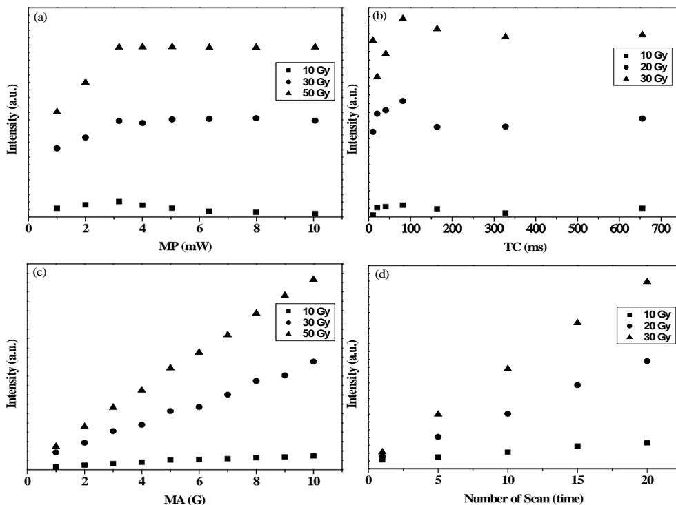
**Fig. 3:** The variation of peak to peak signal intensity with different ESR parameters (a) microwave power (b) time constant (c) modulate amplitude and (d) number of scan
