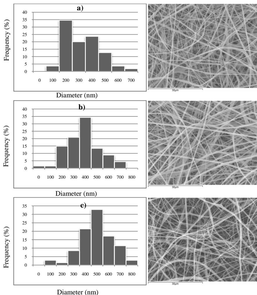
**Fig. 2:** Diameter distribution of the electrospun PVDF nanofibers with concentration a) 11 wt.% b) 13 wt.% c) 15 wt.%
