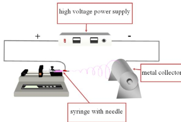
**Fig. 1:** Scheme of an electrospinning equipment.
