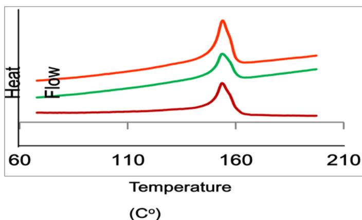
**Fig. 4:** DSC thermograms of the electrospun PVDF nanofibers a) 11 wt.% b) 13 wt.% c) 15 wt.%
