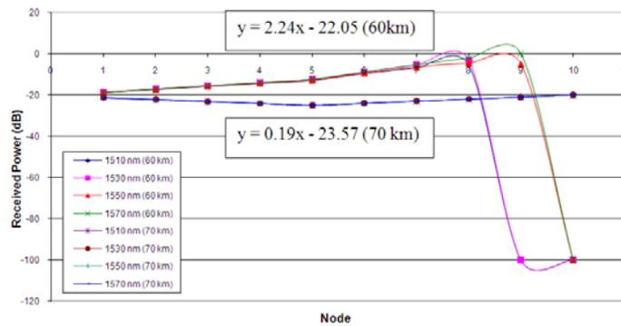
**Fig. 3:** Output power measured at 2.5 Gbps data transmission rate of the distance between two nodes 60 km and 70 km.
