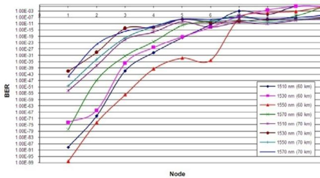
**Fig. 4:** BER performance at 2.5 Gbps data transmission rate of the distance between two nodes 60 km and 70 km.
