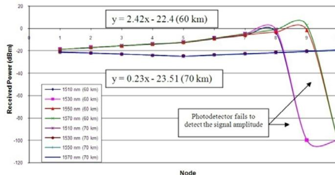
**Fig. 1:** Output power measured at 622 Mbps data transmission rate of the distance between two nodes 60 km and 70 km.
