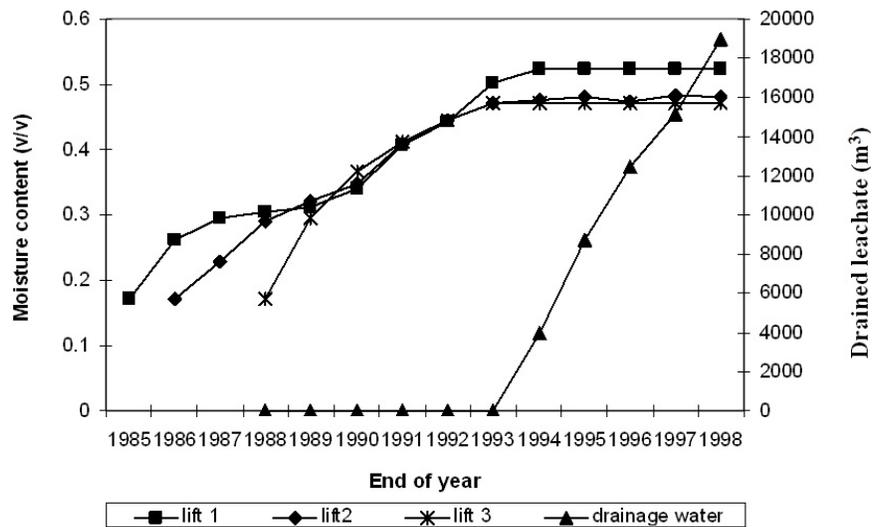
**Fig. 11:** Moisture stored and drained in the landfill incorporating daily cover of 7.5% initial waste layer depth.
