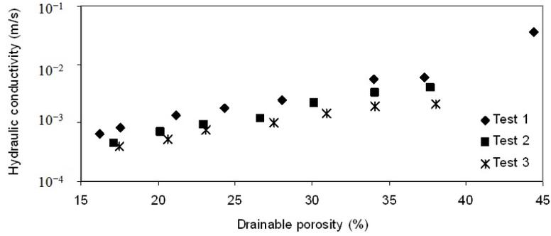
Fig. 6: Saturated hydraulic conductivity of waste fills at various drainable porosities
