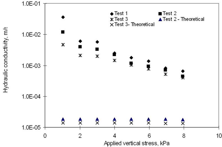
Fig. 7: Saturated hydraulic conductivity of the waste fills at various overburden stresses
