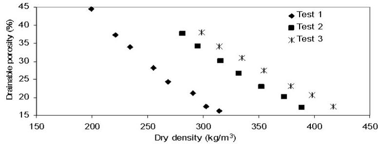
**Fig. 4:** Drainable porosity of the waste fills at various dry densities
