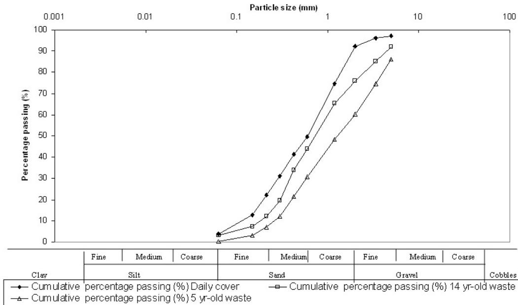
Fig. 2: Particle size distribution curves of the cover soil and fines (<10mm) in the waste samples.
