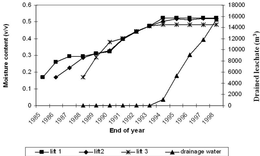
Fig. 12: Moisture stored and drained in the landfill incorporating daily cover of 10% initial waste layer depth.
