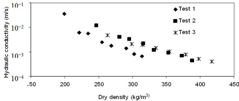
**Fig. 5:** Saturated hydraulic conductivity of waste fills at various dry densities.
