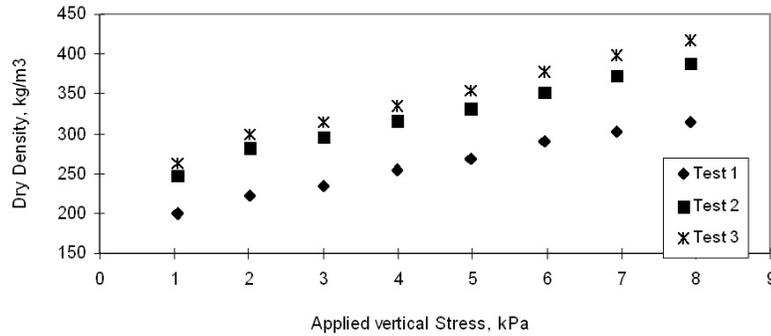
**Fig. 3:** The dry density of the waste fills at various applied
