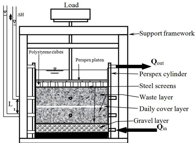
Fig. 1: Schematics of the test cell
