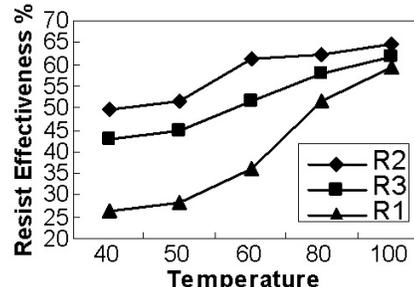
**Fig. 3:** the effect of the temperature on Resist effectiveness of auxiliaries (R<sub>1</sub>,R<sub>2</sub>,R<sub>3</sub>), conditions : pH 4, time 40 min.dye conc. 3%, conc. of salt 1% and conc. of auxiliaries 4%.
