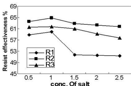
**Fig. 5:** The effect of conc. of salt on Resist effectiveness of auxiliaries ( $R_1$ ,  $R_2$ ,  $R_3$ ), conditions: pH 4, temperature 100 °C, time 40 min., dye conc. 3 % and conc. of auxiliaries 4%.
