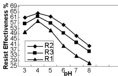
**Fig. 2:** The effect of pH on resist effectiveness of auxiliaries (R<sub>1</sub>, R<sub>2</sub>, R<sub>3</sub>), conditions: temperature 100 °C, time 40 min., dye conc. 3%, conc. of salt 1% and conc. of auxiliaries 4%.
