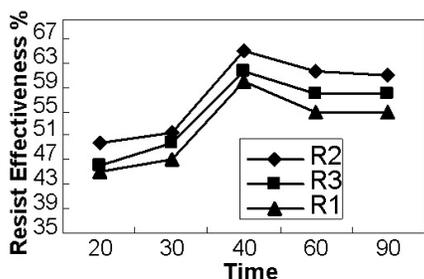
**Fig. 4:** The effect of time on Resist effectiveness of auxiliaries ( $R_1$ ,  $R_2$ ,  $R_3$ ), conditions: pH 4, temperature 100 °C, dye conc. 3 %, conc. of salt 1% and conc. of auxiliaries 4%.
