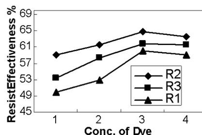
**Fig. 6:** the effect of the conc. of dye on Resist effectiveness of auxiliaries ( $R_1$ ,  $R_2$ ,  $R_3$ ), conditions: pH 4 temperature 100 °C, time 40 min., conc. of salt 1% and conc. of auxiliaries 4%.
