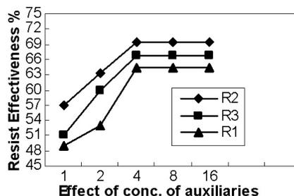
**Fig. 7:** The effects of conc. of auxiliaries on Resist effectiveness of auxiliaries ( $R_1$ ,  $R_2$ ,  $R_3$ ), conditions: pH 4, time 40 min., temperature 100 °C, conc. of salt 1% and dye conc. 3% of acid red 27.
