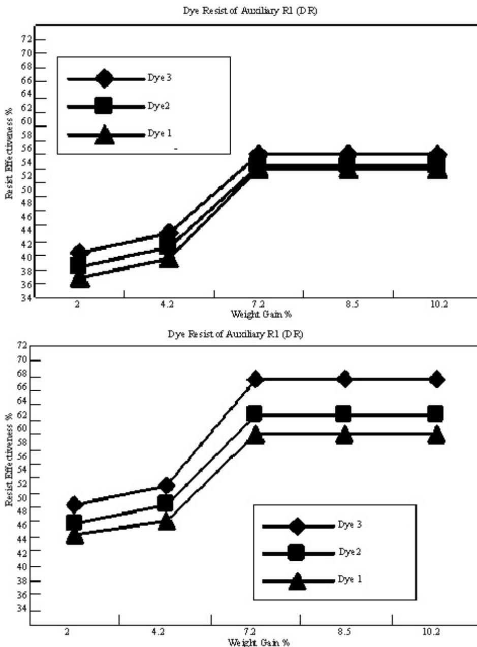
Fig. 10a,b: Resist effectiveness of  $R_1$  versus auxiliary uptake of the fibres
