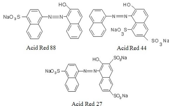
Fig. 1: Dye structures.
