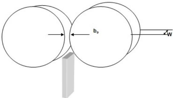
**Fig. 2:** A sheet of width  $W$  and thickness  $b_0$  is produced according to the minimum gap and rolls' width respectively
