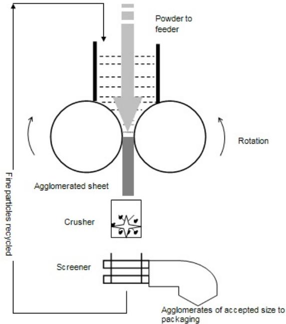
**Fig. 1:** Agglomeration process using roll press machine
