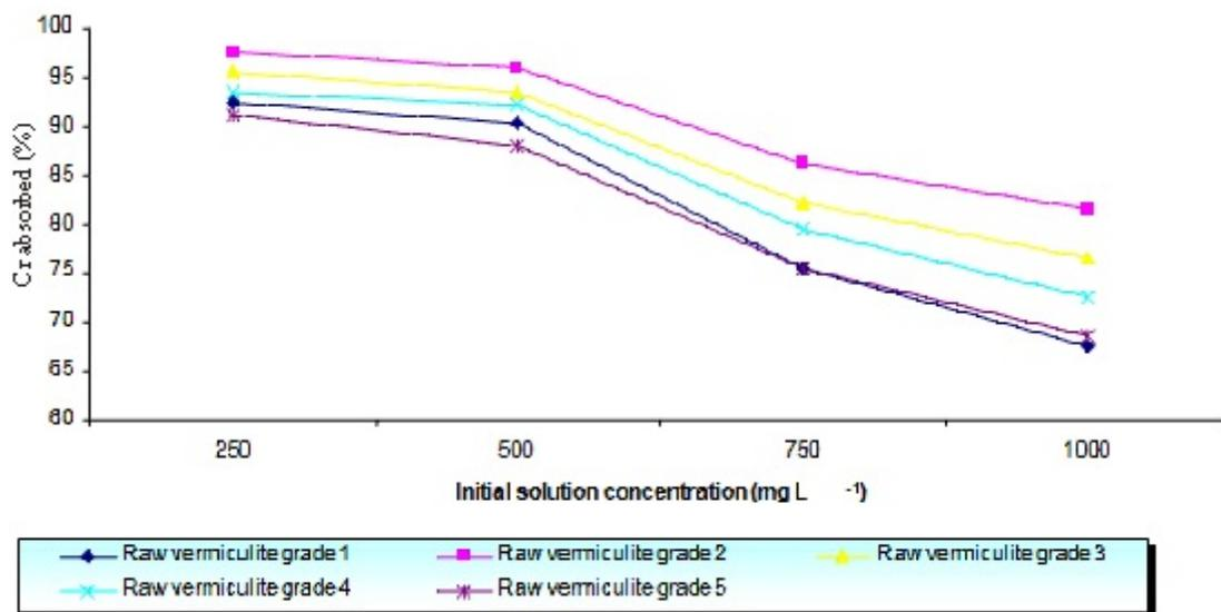
Fig. 2: Absorption of Cr on raw vermiculite grades (1 to 5) as a function of initial solution concentration.
