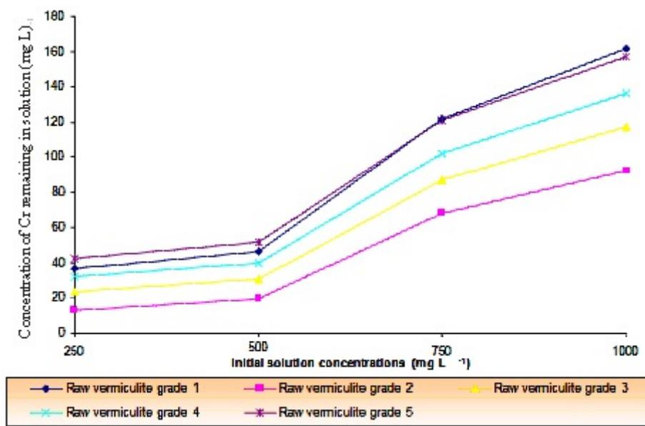
**Fig. 1:** Adsorption of Cr as a function of initial solution concentration for raw vermiculites grade (1 to 5).
