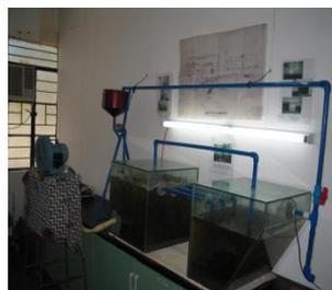
The Biofermenting Machine which is core of the study is photographed on different perspectives. The said machine is aimed to treat wastewater, production of solid sludge for fertilizer and production of spirulina
