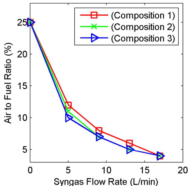
**Fig. 4:** Variation of air to fuel ratio with syngas flow rate at 1200 rpm.
