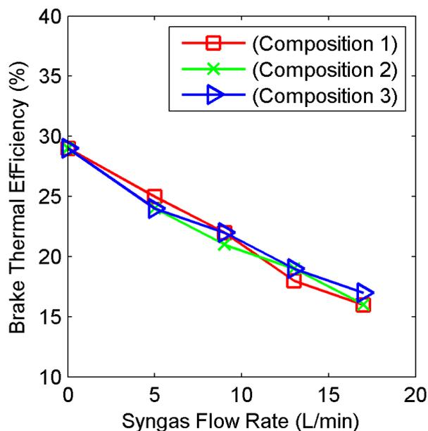
**Fig. 5:** Variation of brake thermal efficiency with syngas flow rate at 1200 rpm.
