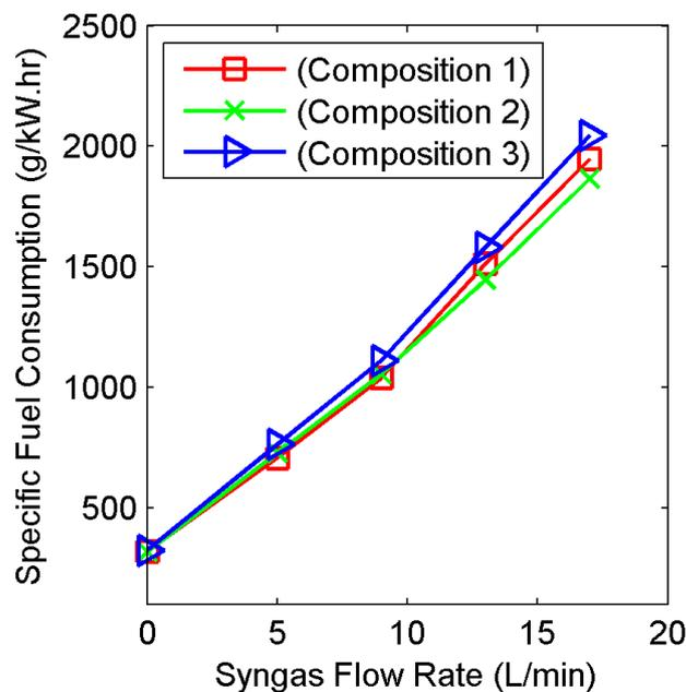
**Fig. 3:** Variation of specific fuel consumption with syngas flow rate at 1200 rpm.
