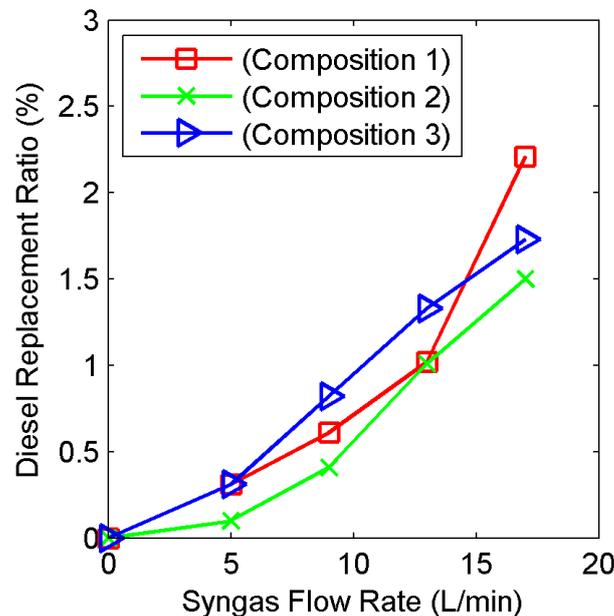
**Fig. 6:** Variation of diesel replacement rate with syngas flow rate at 1200 rpm.
