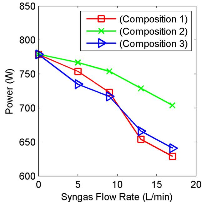
**Fig. 2:** Variation of brake power with syngas flow rate at 1200 rpm.
