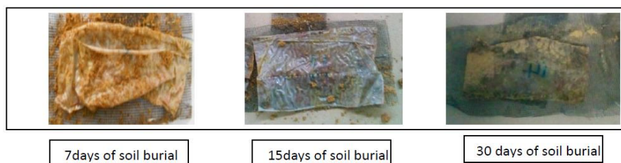
Fig. 1: Visual Analysis of PVOH:Starch 50:50 in 18% of soil moisture content.
