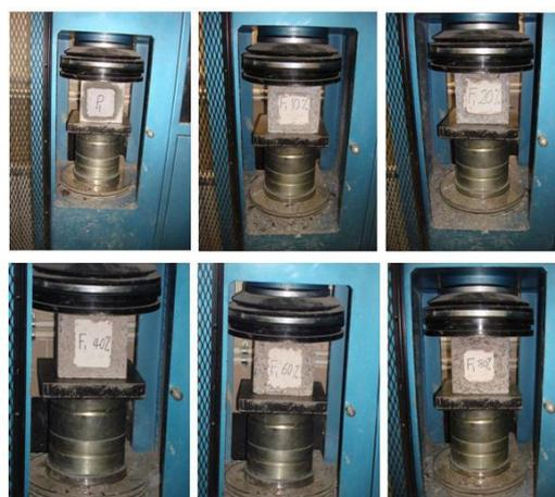
**Fig. 3:** Loading of cubic specimens with a percentage of 0, 10, 20, 40, 60 and 80, by total weight of the fine aggregate in concrete.
