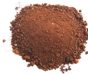
**Fig. 1:** Sample of Incinerator Ash.
