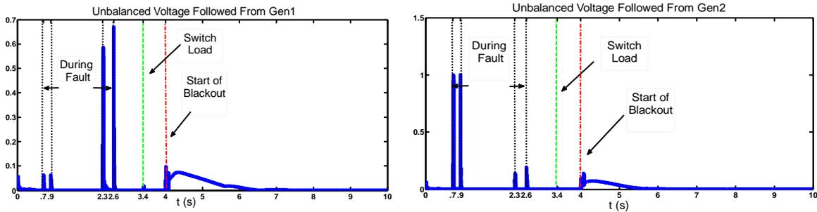
Fig. 7: UV measured from Gen1, Gen2 terminal.
