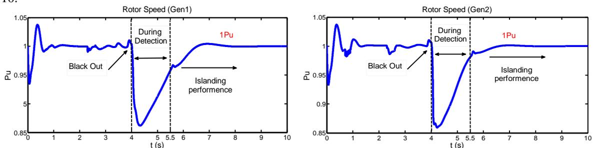
Fig. 10: Rotor speed of distributed generation Gen1, Gen2 under conditions apply.
