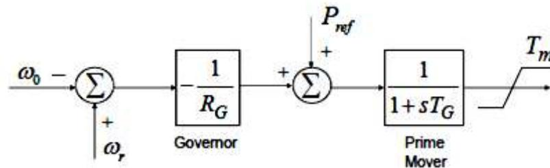
**Fig. 2:** Schematic of the governor.
