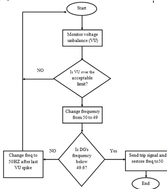
**Fig. 3:** Simplified algorithm for islanding detection.
