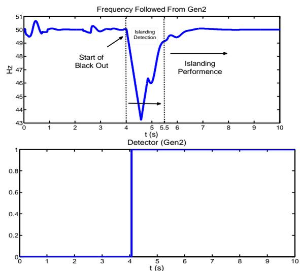
Fig. 9: Frequency and detecting the time of islanding
