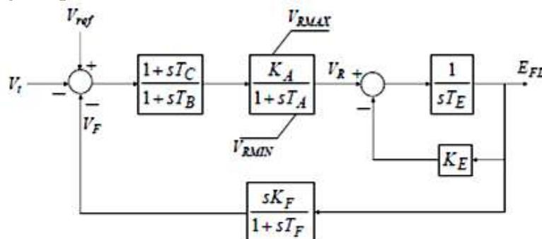
**Fig. 1:** Schematic of the exciter system.
