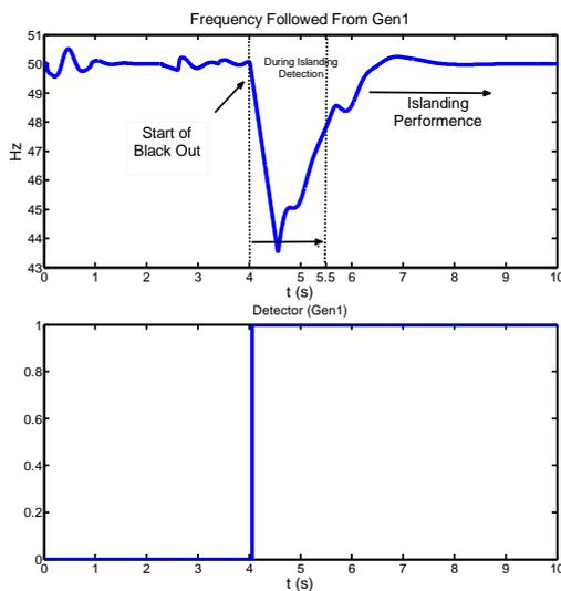
Fig. 8: Frequency and detecting the time of islanding
