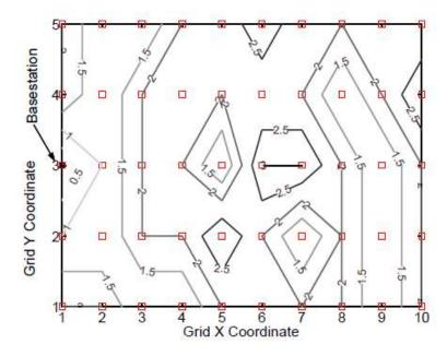
Fig. 5: Average Hop over Distance Contour Plot for MT at power 70 for the indoor 50-node deployment.
