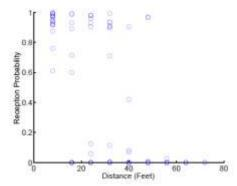
**Fig. 3:** Indoor reception probability of all links of a network in a line topology at low transmit power setting (70) in the fover.
