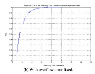
**Fig. 8:** Empirical cumulative distributive functions of the parent switching cost differenceof a 21-node network under congested load, with and without the overflow error.
