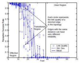
**Fig. 1:** Reception probability of all links in a network, with a line topology on a tennis court. Note that each link pair appears twice to indicate link quality in both directions.
