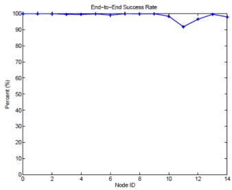
Fig. 7: End-to-end success rate of MT on Mica2 deployed in an office environment.
