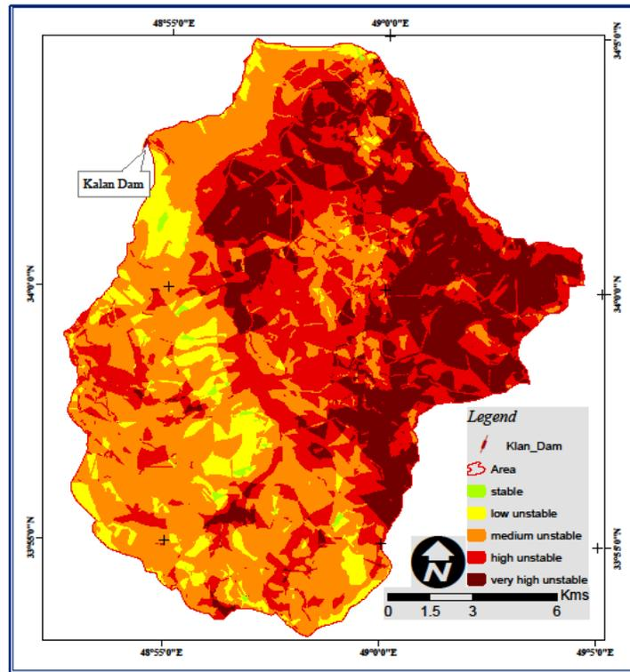
**Fig. 8:** zonation map with the stability slope movement in Kalan dam basin
