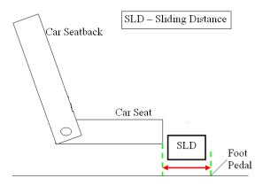
Fig. 1: Car seat horizontal adjustment measurement.
