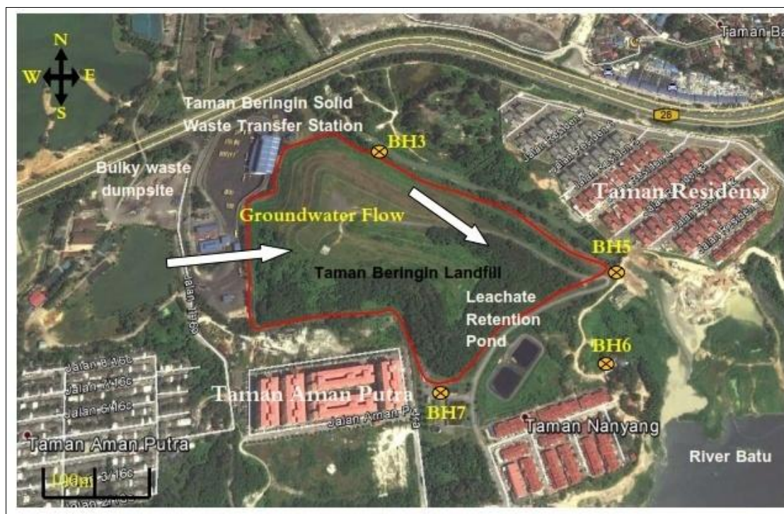
Fig. 1: Taman Beringin Landfill (TBL) site and the position of groundwater monitoring wells.
