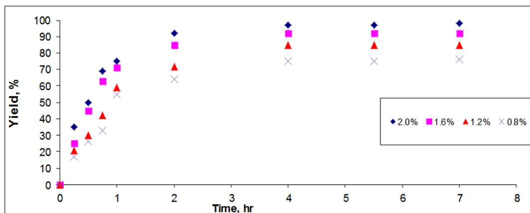
Fig. 3: Effect of catalyst - 15 % of n-hexane.
