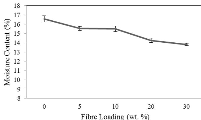
**Fig. 3:** The moisture content of starch-kenaf biocomposite.
