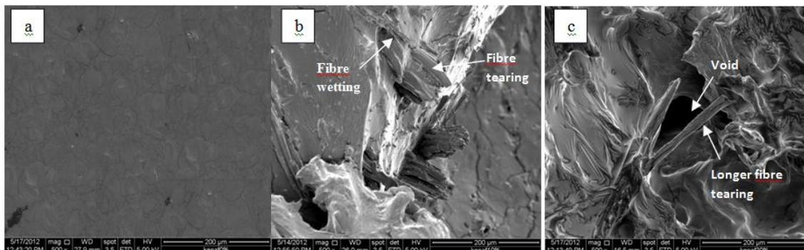
**Fig. 2:** SEM images of starch reinforced kenaf fibre biocomposite at (a) 0 wt.%, (b) 10 wt.% and (c) 30 wt.% of kenaf fibre content.
