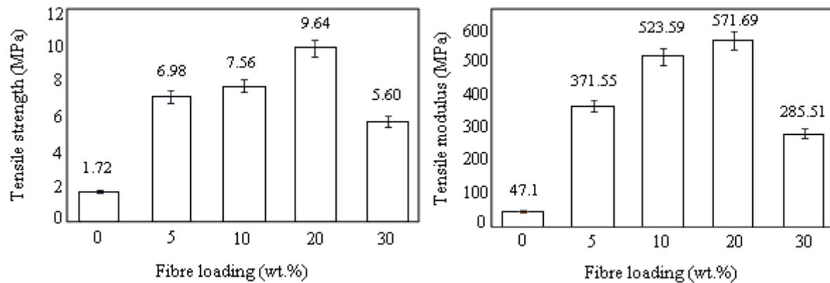
**Fig. 1:** Tensile properties of the starch-kenaf biopolymer composite.
