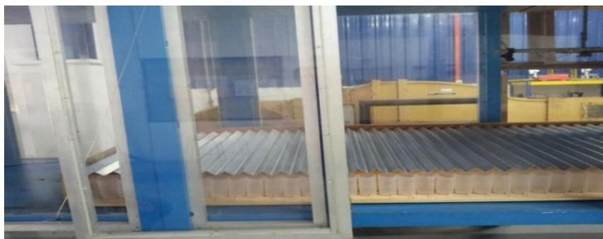
**Fig.1:** Experimental setup in the wind tunnel to determine spray drift from flat fan nozzle TP. Patternator 300 cm length  $\times$  100 cm width spray table with fifty V-shaped gutters (6 cm width  $\times$  3 cm depth).
