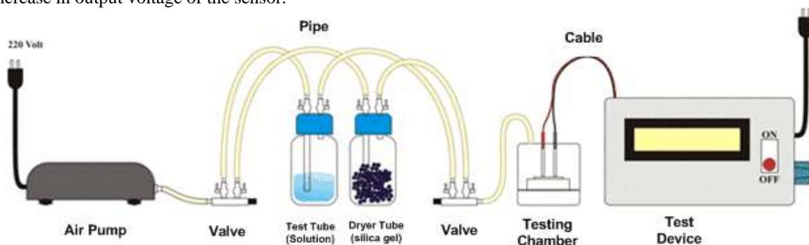
**Fig. 2:** Electrical testing of sensor properties scheme.
