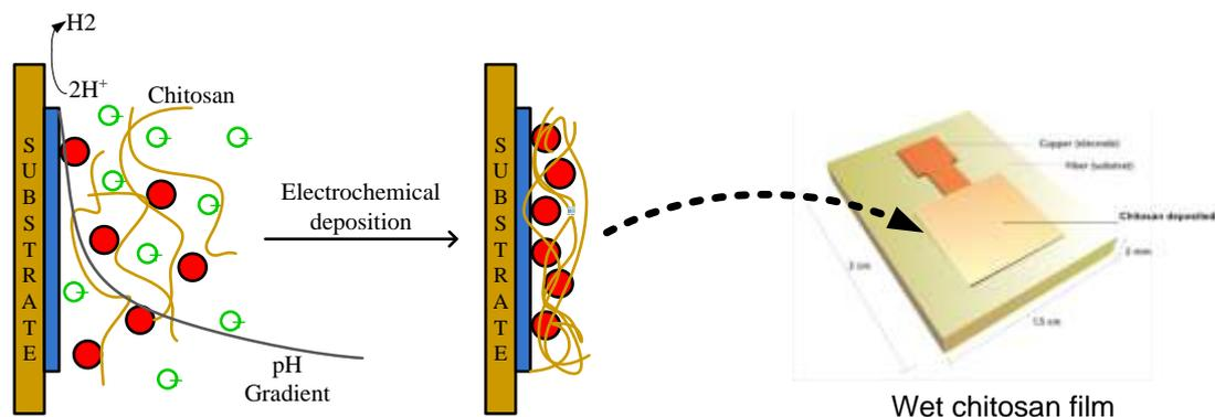
**Fig. 1:** Chitosan coating process with electrochemical deposition method
