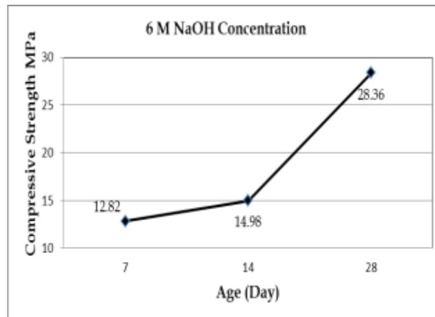
Fig. 8: Compressive strength results with 6 M.
