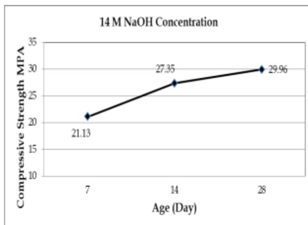
**Fig. 12:** Compressive strength results with 14 M.
