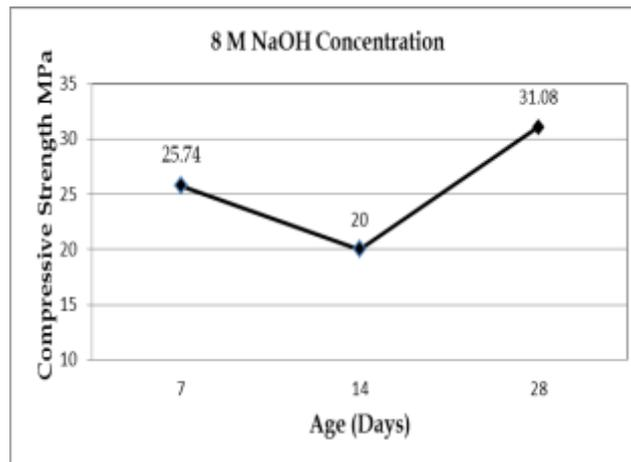
Fig. 9: Compressive strength results with 8 M.
