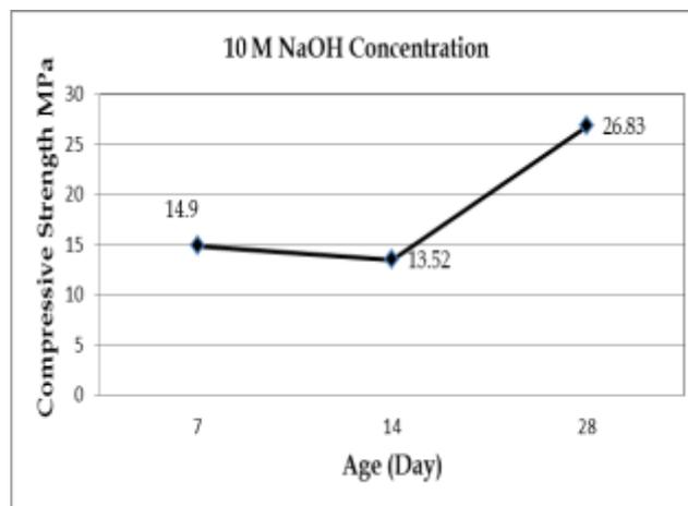
Fig. 10: Compressive strength results with 10 M.
