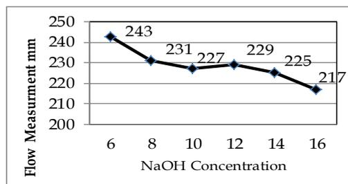
**Fig. 1:** Flow measurement verses sodium hydroxide concentration.
