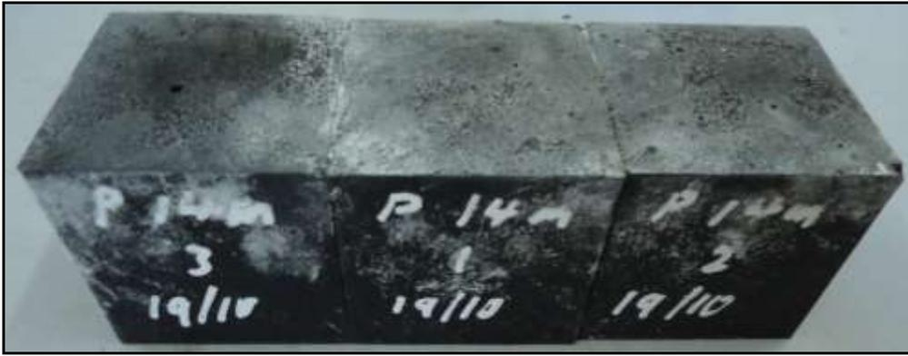
Fig. 6: Efflorescence.
