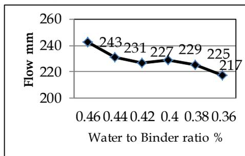
**Fig. 2:** Flow measurement verses water to binder ratio.
