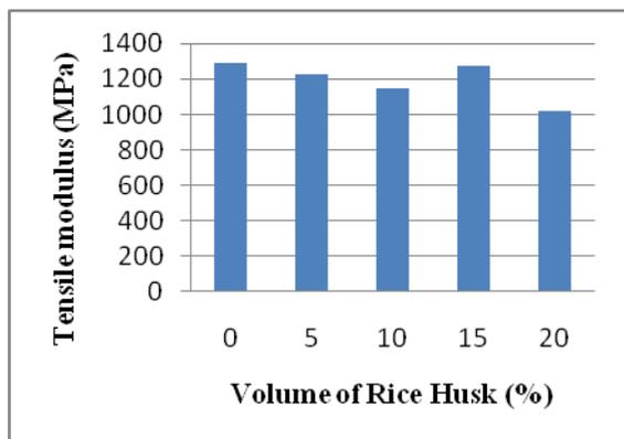
**Fig. 5:** Effect of rice husk volume fraction on tensile modulus
