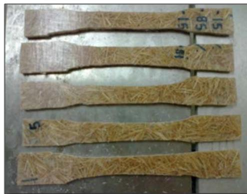
**Fig. 2:** Tensile specimen Each value obtained represented the average of five samples.
