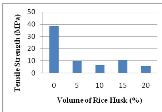
**Fig. 4:** Effect of rice husk volume fraction on tensile strength
