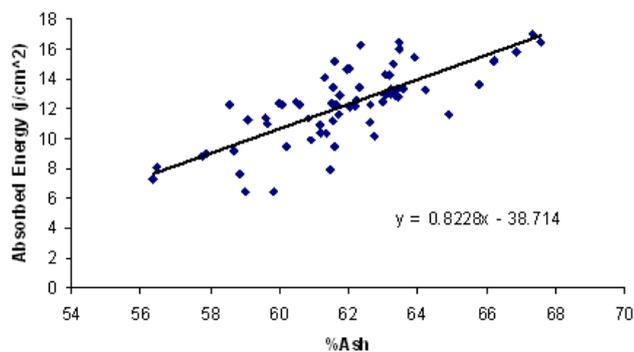
**Fig. 6:** The graph of impact energy absorbency changes with ash percentage which shows that as ash percentage increases the amount of energy absorbency increases too.
