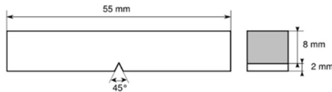
**Fig. 2:** The size of sample in order to impact test of Charpy according to ASTM E26 standards.
