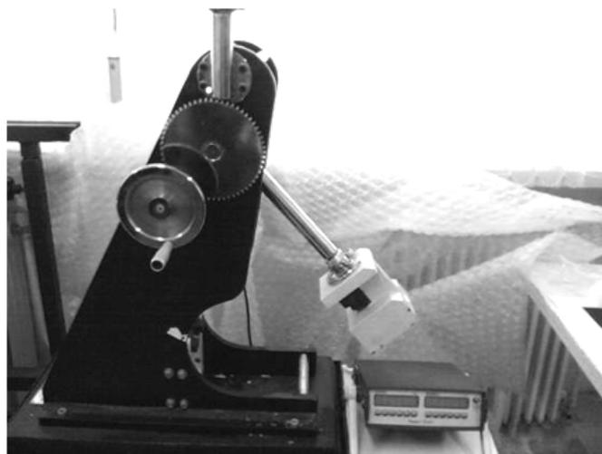
**Fig. 3:** Charpy impact tester in biomechanics laboratory.
