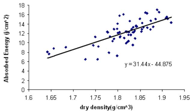
**Fig. 4:** The graph of impact energy absorbency changes with dry density which shows that as density increases the energy absorbency increases too.
