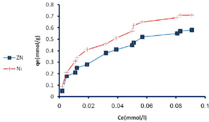
Fig. 3: Sorption isotherm of nickel and zinc ions in deionized water.
