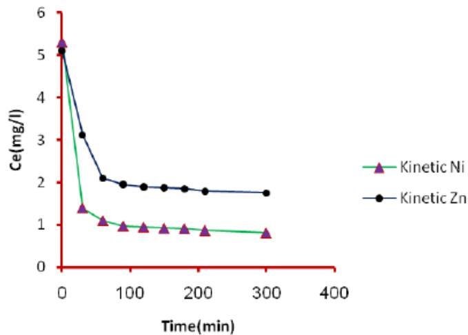
Fig. 4: The adsorption kinetic of nickel and zinc ions at pH 5.5 and 25°C in deionized water
