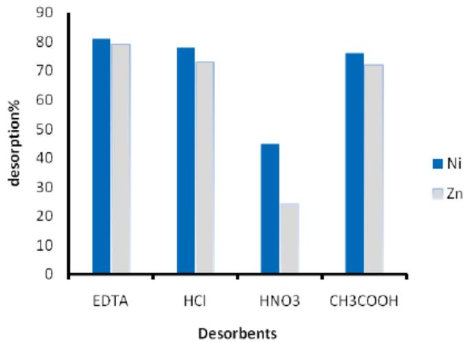
Fig. 2: Nickel and zinc ions recovered by different desorbents 6
